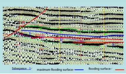
Fig2 Stratigraphic sequence seismic section
